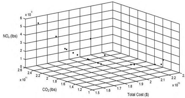
Figure 1: Tradeoff between planning cost and air emissions [14]
